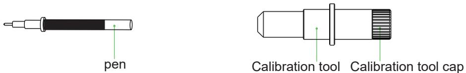
(1) First, unscrew the Calibration tool cap, as shown.
