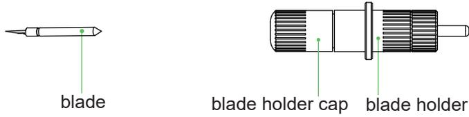
(1) First, unscrew the blade holder cap, as shown.
