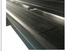
**Special paper-press device:** it can press broadside of the paper, avoid any rubbing with paper during the moving of vehicle.
