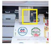
**Red light positioning system:** with the assistance of red light positioning system, it can sense the printed mark point to realize accurate contour cutting automatically.
