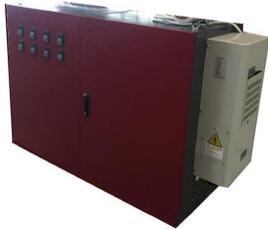
A photograph of a red control cabinet with a white air conditioner unit attached to its side, used for temperature control in tropical areas.                | <b>Control cabinet with air conditioner:</b> the air conditional installed on the control cabinet, ensure the machine can be used in tropical area countries to reduce the temperature inside of the cabinet, avoid damage of the electric components. |
