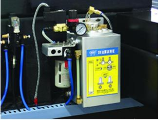
A photograph of a mist sprayer cooling system, which is a yellow and blue unit with various hoses and gauges, used for spraying mist to tools during cutting. | <b>Mist sprayer Cooling System:</b> Use alcohol or other coolants to spray mist to the tools during cutting, which makes the cutting edge smoother and cool down the cutting tools.                                                                    |
